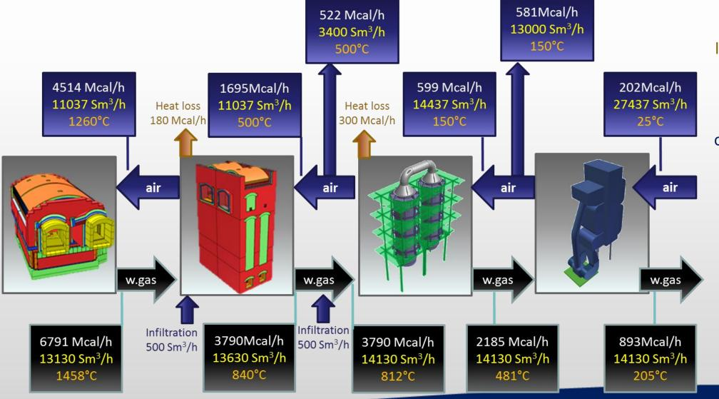
In order to optimize the thermal exchange in lower temperature zones, it is usual to add a convective heat exchanger to the radiating ones. This kind of component guarantees a high efficiency at low thermal levels and a noticeable design flexibility, and its physiological stops for maintenance and cleaning, thanks to a proper bypass system, penalize the plant efficiency only for a few percent point, commonly for a few days a year.
